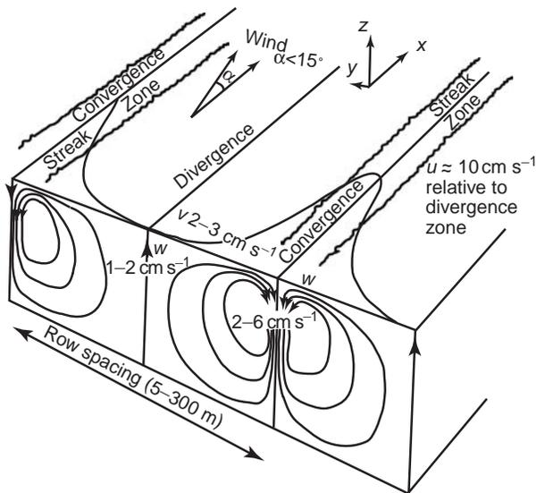
**Figure 7** Langmuir cells and the associated velocities. Note the “windrows” and the strong near-surface vertical velocities associated with the convergence zones of a pair of counter rotating cells. Note the zones indicated as streak zones are the ‘windrows’.  $\alpha$  is the angle between the wind and the windrows,  $w$  is the vertical velocity,  $u$  and  $v$  are velocities in the  $x$  and  $y$  directions. (Kantha and Clayson, 2000.)
