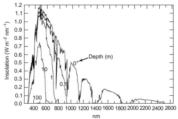
**Figure 4** Solar insolation at the ocean surface and below. Note the rapid attenuation of nonvisible components with depth. Only the visible part remains below about 10 m. (Kantha and Clayson, 2000.)
