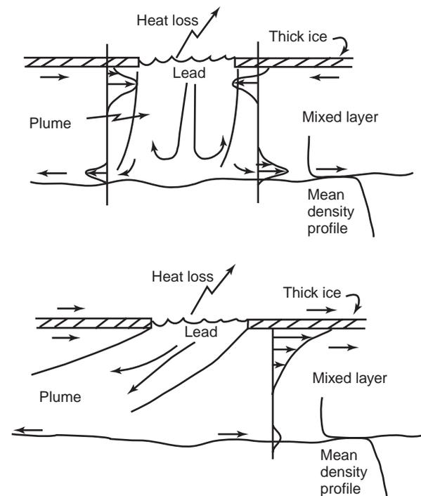
**Figure 2** OML driven by freezing and salt extrusion underneath a refreezing lead. The top panel corresponds to stationary ice cover, when free convection dominates, and the bottom panel to the case when the ice is in motion, when forced convection dominates the mixing process. (Kantha and Clayson, 2000.)
