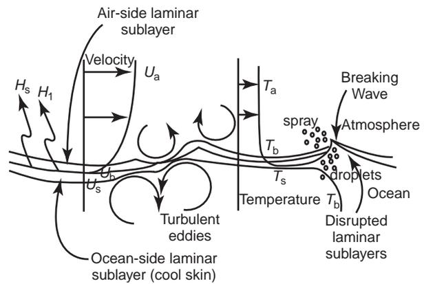
**Figure 6** A sketch of the air–sea interface showing the molecular sublayers on the air and the water sides. The heat flux through the sublayer on the water side is responsible for the large temperature gradient there and hence the cool skin of the ocean. (Kantha and Clayton, 2000.)
