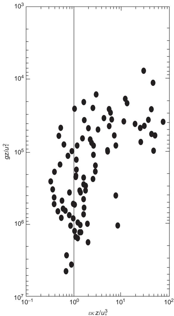
**Figure 3** Measured dissipation rate of TKE in the near-surface layers of the OML. The dissipation rate is more than an order of magnitude higher than that expected from the classical law of the wall scaling.  $g$  is the gravitational acceleration and  $\kappa$  is the von Karman constant. (Kantha and Clayson, 2000.)
