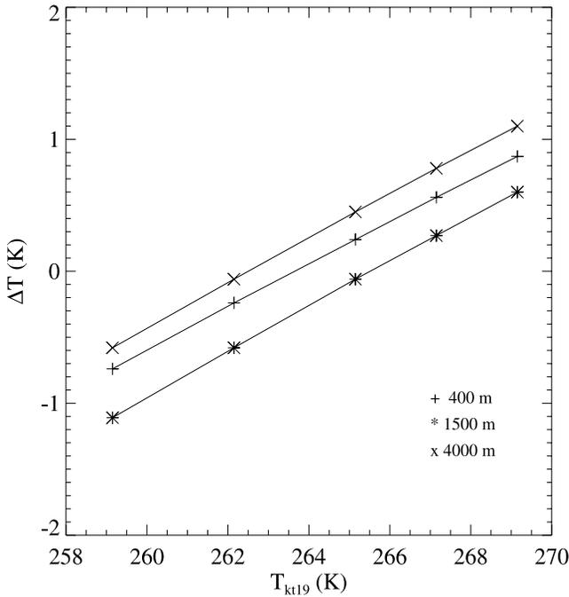
**Figure 1.** Corrections applied to KT19 brightness temperature measurements to account for atmospheric radiance and emissivity effects. Data shown are for 20 May 1998 at three flight altitudes.
