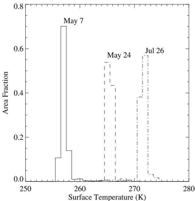
**Figure 5.** Distribution of surface temperatures over a 30 km box surrounding the SHEBA ice station for 7 and 24 May and 26 July 1998.
