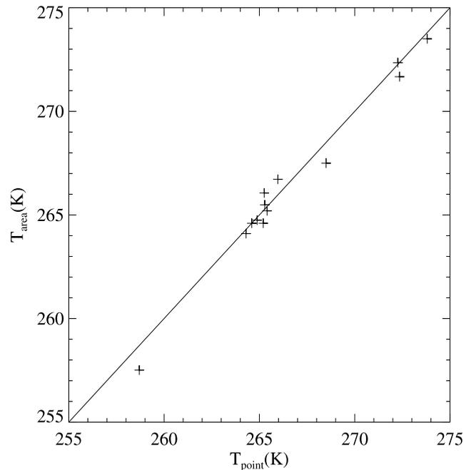
**Figure 6.** Comparison of KT19 surface temperatures at the SHEBA site (“point” measurement) with mean values over the C-130 flight patterns (“area” measurement).
