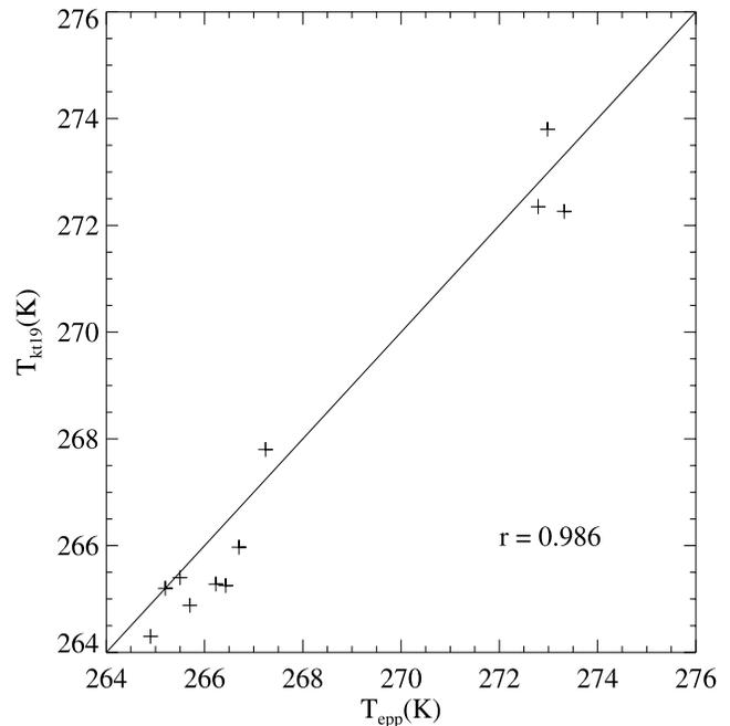
**Figure 4.** Comparison of surface temperature derived from the KT19 with ground-based Eppley measurements for cases where the C-130 overflew the SHEBA ice station.
