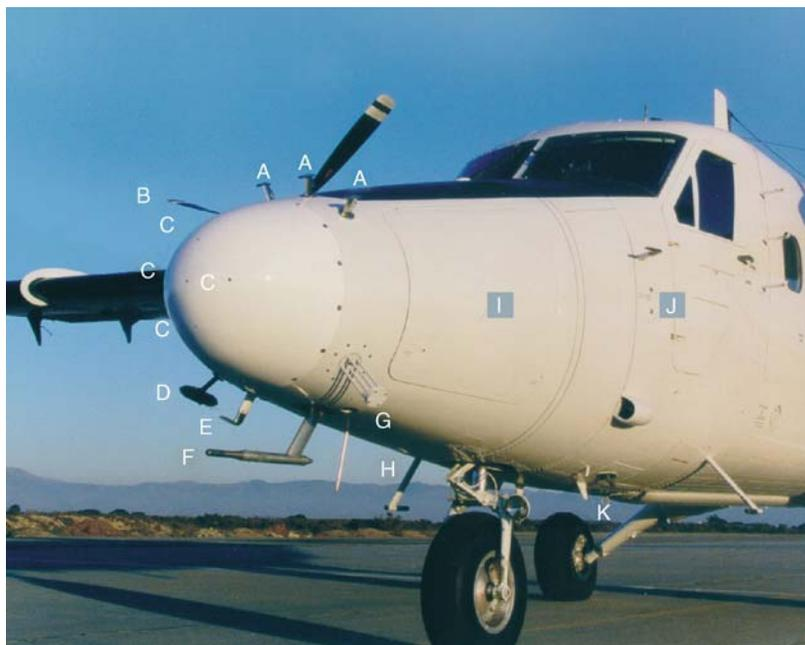
**Figure 4** A Twin Otter research aircraft operated by the US Department of the Navy, equipped with sensors to study wind, temperature, and humidity structure in the atmospheric boundary layer (Photo: © Carl Friehe.)
