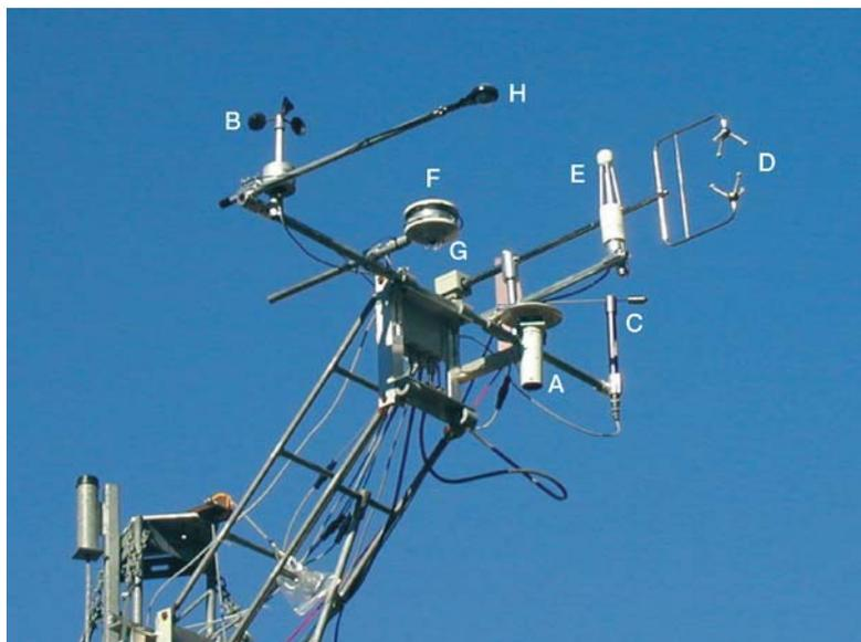
**Figure 1** An array of meteorological research instruments at the top of a 30 m tower, part of the ‘Ozflux’ long-term climate monitoring network in Australia. (Photo: ©Frank Bradley.)
