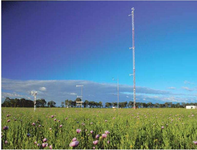
**Figure 2** A micrometeorological research site in south-eastern Australia, set up by CSIRO Land and Water. The towers carry instruments to measure the profiles of wind, temperature, and humidity, the components of radiation, and eddy fluxes of heat, moisture and  $\text{CO}_2$ , as part of a regional climate study. The tallest tower is 22 metres high; a shelter for recording equipment is seen to the right of the picture. (Photo: ©Greg Heath.)
