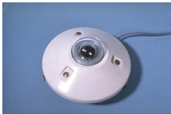
Figure 1 A pyranometer used for measuring short-wave radiation. The thermopile is covered by two transparent domes. (Photograph courtesy of Southampton Oceanography Centre.)
