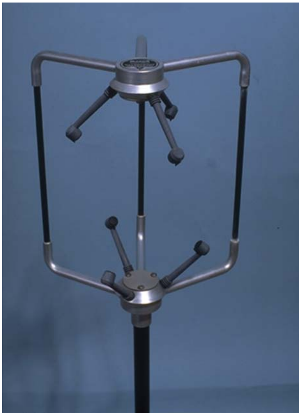
Figure 2 The sensing head of a three-component ultrasonic anemometer. The wind components are determined from the different times taken for sound pulses to travel in either direction between the six ceramic transducers. (Photograph courtesy of Southampton Oceanography Centre.)
