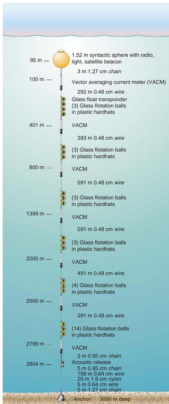
**Figure 1** A typical subsurface mooring design. (Design by S. Worriolow.)
