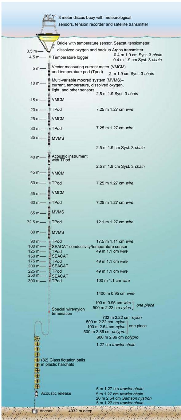
**Figure 3** An inverse catenary mooring design. (Design by G. Tupper.)
