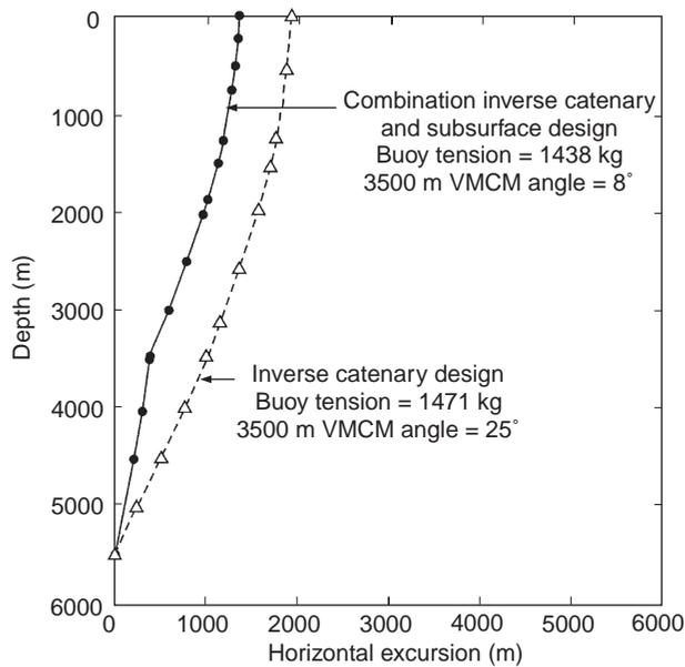
**Figure 6** A comparison of the shapes of two mooring designs subjected to the same ocean current forcing, showing the differences in mooring inclination at 3500 m depth.
