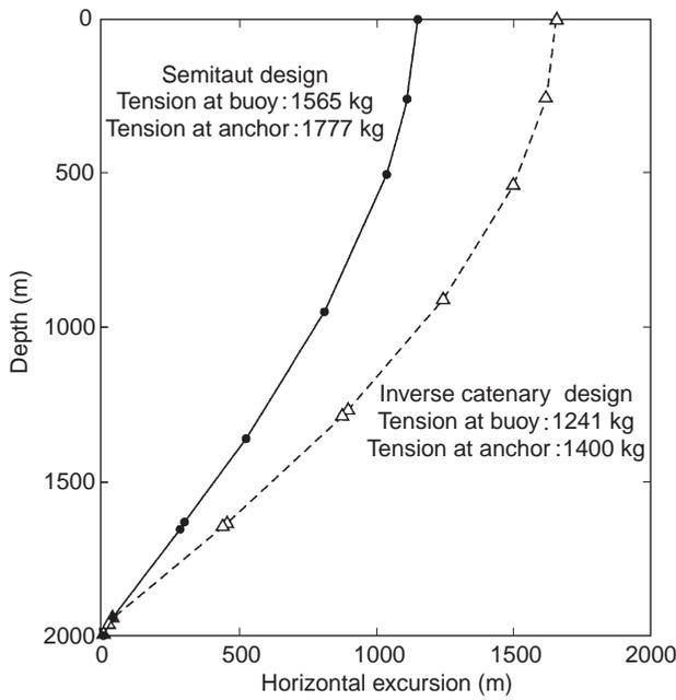
**Figure 4** A comparison of the shape of a semitaut design with that of an inverse catenary design when subjected to the same ocean current forcing. Note the differences in buoy and anchor tensions as well as the horizontal excursions at the surface.
