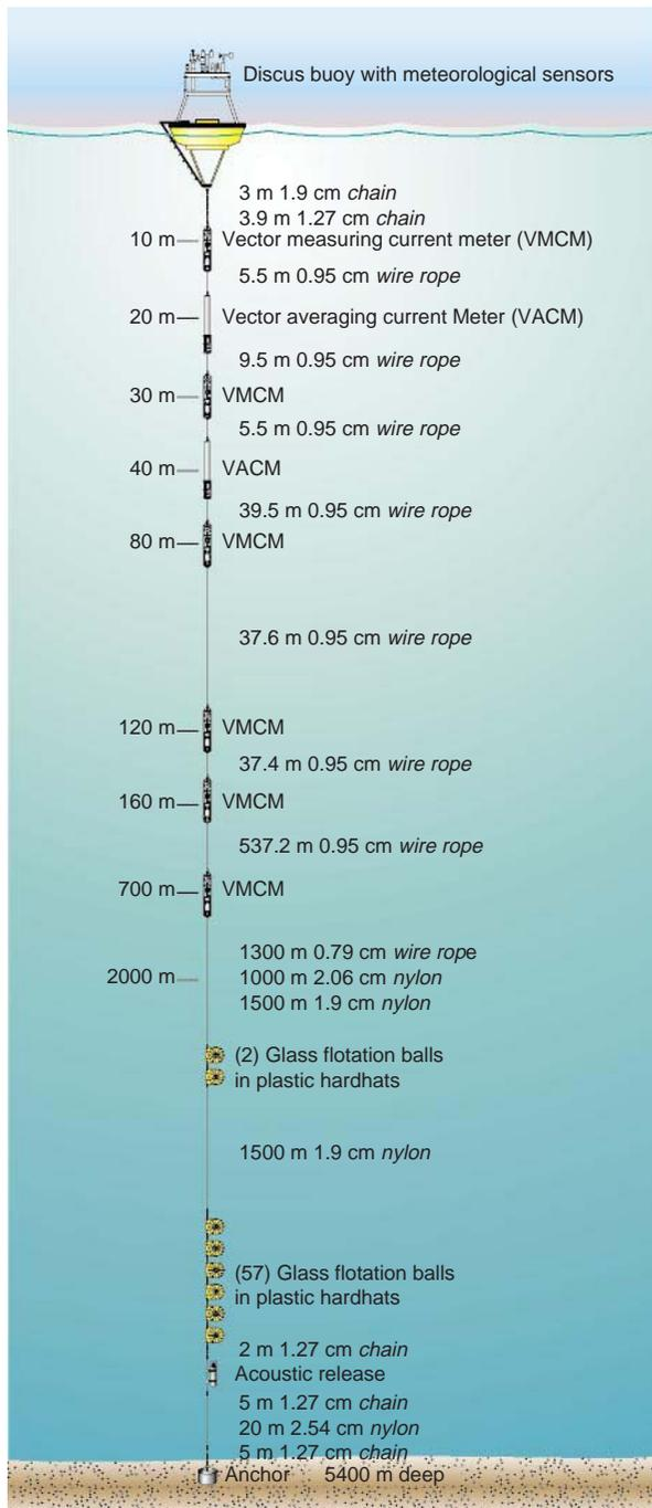
**Figure 2** A semitaught surface mooring design. (Design by P. Clay.)
