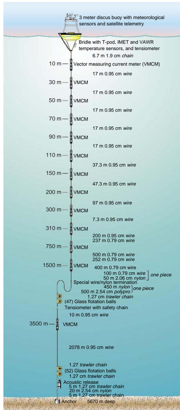
**Figure 5** A mooring design that combines the features of an inverse catenary mooring with those of a semitaut mooring in order to improve the quality of deep (3500 m) current measurements made from a surface mooring. (Design by G. Tupper.)
