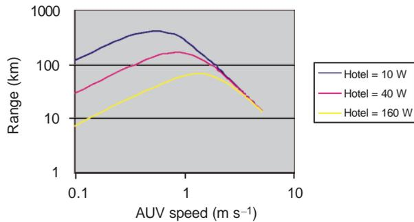
**Figure 2** Range as a function of hotel load and speed. These calculations were made for a low drag 2.2 m long, 0.6 m diameter vehicle with high efficiency propulsion and batteries providing  $3.3 \text{ kW} \cdot \text{h}$  of energy
