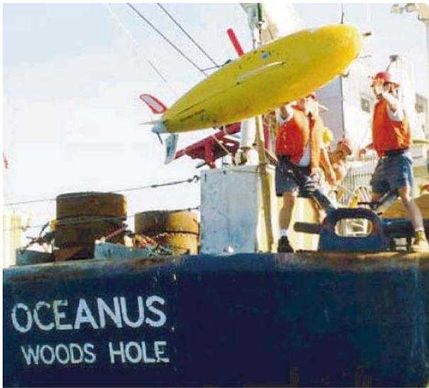
**Figure 1** An Odyssey class AUV being deployed from the stern of the R/V *Oceanus*.
