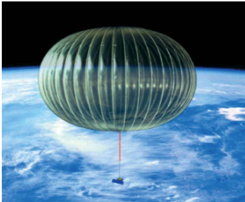
**Figure 7** Artist's view of the ULDB pumpkin super-pressure balloon at float. Designed for carrying one tonne at 35 km altitude during 100 days, such balloons could allow the remote sensing of the atmosphere on a global scale at far less cost than that of using satellites. © NASA.
