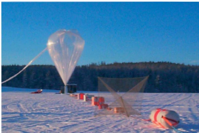
**Figure 4** Small, light, zero-pressure balloon of 10 000  $\text{m}^3$  ready for launch at the ESRANGE facility at Kiruna in northern Sweden during the Ozone THESEO-SOLVE campaign in February 2000. Five complementary scientific instruments for measuring chemicals and aerosols by a variety of techniques are shown ready to be flown together in separate packages which at launch slip along the launch pad. © CNRS.
