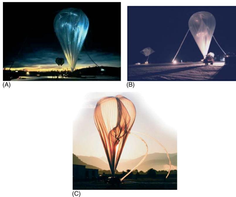
**Figure 2** (A) + (B) Inflation of a 100 000 m<sup>3</sup> zero-pressure balloon in the polar night in northern Sweden in January 2000 for studying stratospheric clouds and ozone depletion. The two small balloons in the background are auxiliary balloons used to keep the payload off the ground during liftoff. © CNRS. (C) Early-morning inflation of a 100 000 m<sup>3</sup> zero-pressure balloon at Gap in the Alps. © CNES.
