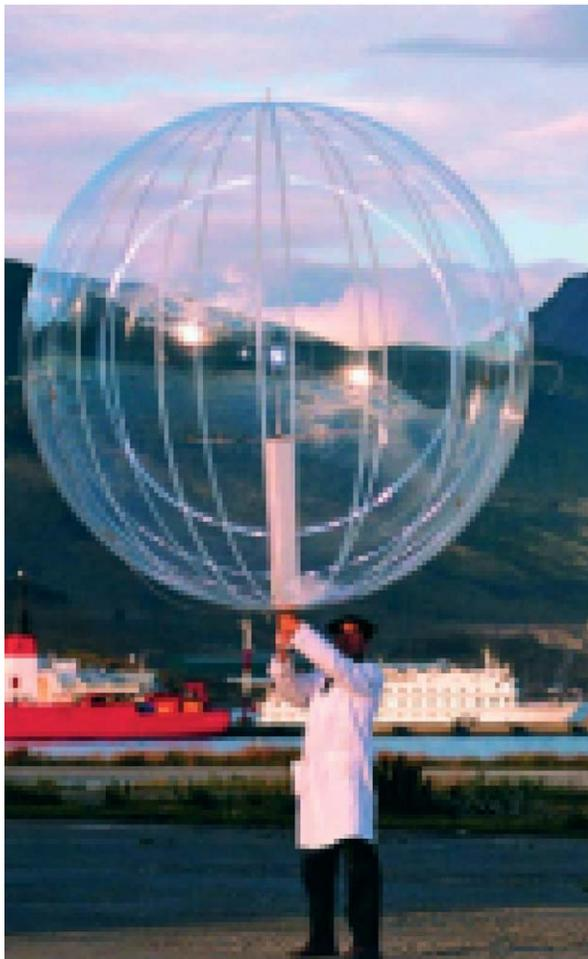
**Figure 5** Launch of a tracer super-pressure balloon at Ushuaia, Argentina, in February 2000 for studying the meteorology of the lower atmosphere over the Southern Atlantic. The electronics are located inside the balloon for protection against rainfall.
