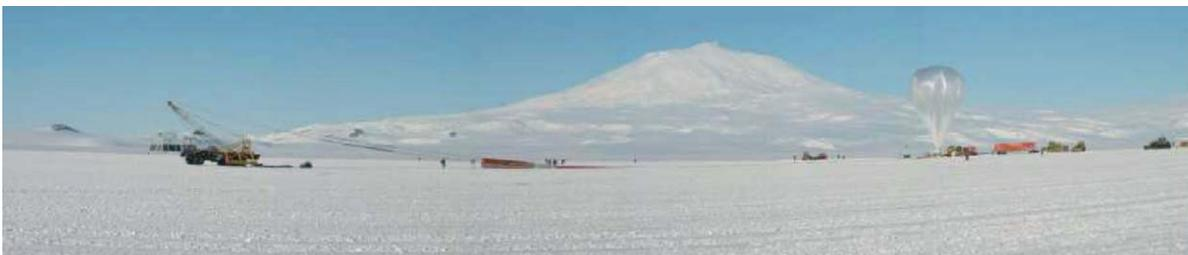
**Figure 3** 1 000 000 m<sup>3</sup> zero-pressure balloon ready for release at MacMurdo, Antarctica, in December 2001. The 1100 kg payload is suspended from a mobile crane. Taking advantage of the polar day, a record flight of one month was achieved. © NASA.
