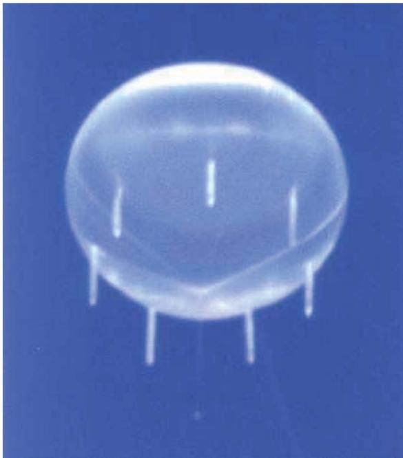
**Figure 1** Zero-pressure balloon of 2 000 000  $\text{m}^3$  at float altitude. The excess gas is vented by seven open ducts at the bottom of the envelope. © NASA.
